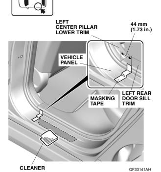
7. Temporarily attach the adhesive backings.
