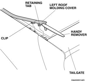
3. Remove the left roof molding.
