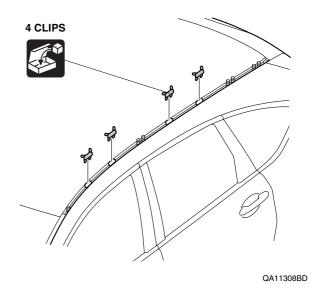
13. Remove the left roof molding cover.
