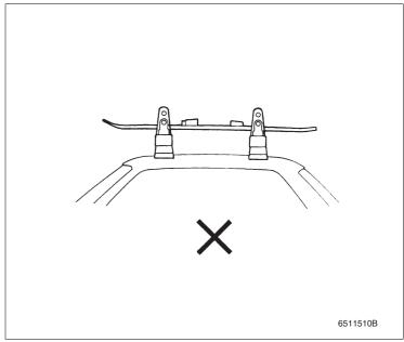
• If the bindings cannot be positioned between the front an rear attachments, install the ski(s) astride the rear attachment as shown.
