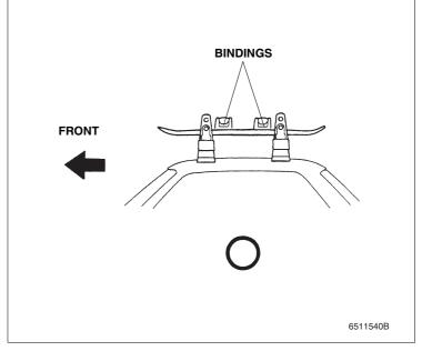
• If the bindings cannot be positioned between the front and rear attachments, install the snowboard astride the rear attachment as shown.
