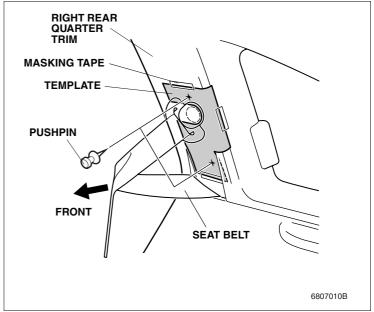
Remove the template, drill holes with an electric drill and 3 mm drill bits at the positions marked in step 2, and then widen the holes to a diameter of 10 mm.
