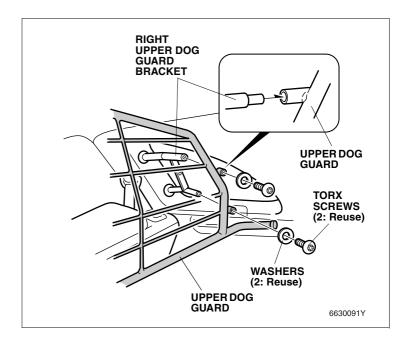
13. Install the upper dog guard anchor to the two grommets installed in step 4.
