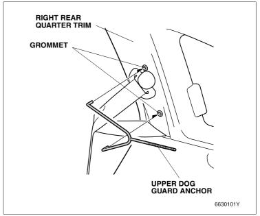
Pass the bolt part of the upper dog guard anchor through the hole of the right upper dog guard bracket.
