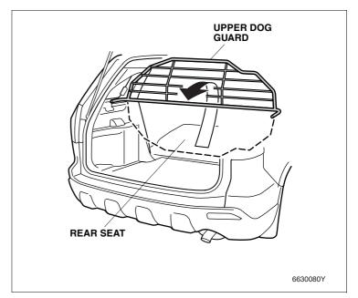
9. Remove the end cap and the knob from the upper dog guard anchor.
