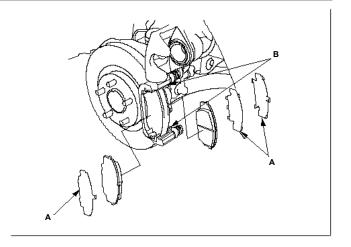
Using vernier calipers, measure the thickness of each brake pad lining. The measurement does not include the pad backing plate (A) thickness.
