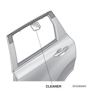
15. Temporarily attach the adhesive backings.
