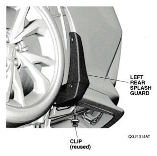
18. Turn the steering wheel fully clockwise. Turn the template over and repeat steps 2 through 17 to install the right splash guards.
