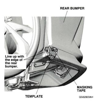
6. Using a felt-tip pen, mark the left rear inner fender along the template.
