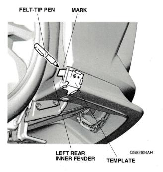
7. Using a pushpin, pierce the center of the two marks on the template.
