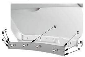
1. Install the tailgate upper trim panel (A). Make sure the hooks (B), the tabs (C), and the clips snap into place securely.
