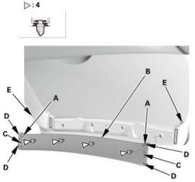
Carefully pry out the notch (A) in the tailgate upper trim (B) with the trim tool to detach the hooks (C) and the tabs (D) from the tailgate side trims (E), and pull back the tailgate upper trim panel by hand to detach the clips, then remove the tailgate upper trim panel.
