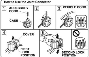
How to deal with the incorrectly secured joint connector. Do not remove the secured joint connector once.
