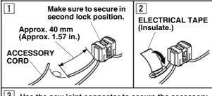
Use the new joint connector to secure the accessory cord to the correct cord.
