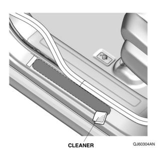
3. Temporarily attach the adhesive backings.
