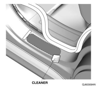
10. Temporarily attach the adhesive backings.
