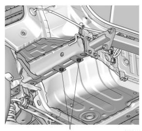
2 BOLTS, 10 x 40 mm (Tighten until they stop, if loose.)
