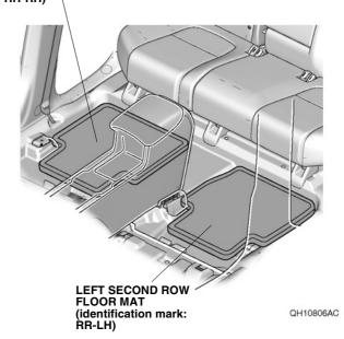
8. Check that all parts are installed properly. (End of installation)
