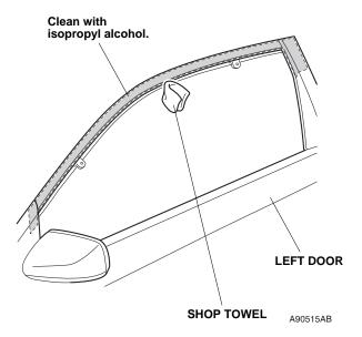
Remove the adhesive backings from one sealer A and one sealer B and attach them to the door sash as shown.
