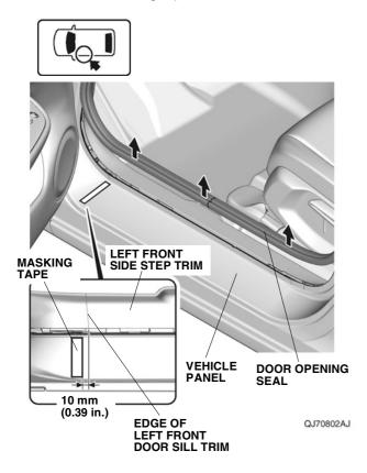
3. Temporarily attach the adhesive backings.
