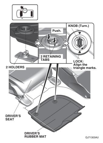
Check that all parts are installed properly. (End of installation)
