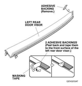
16. Remove the adhesive backing.
