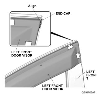
While applying light pressure against the left front door visor, carefully remove the adhesive backings in the order shown. Make sure to push up on the brackets while removing the adhesive backings.
