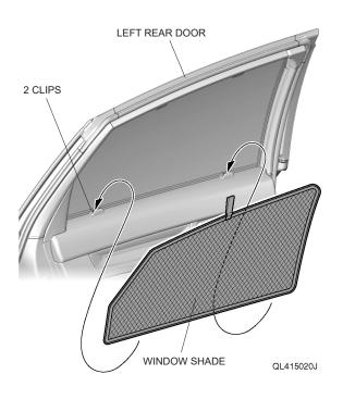
2. Install the top of the window shade into the clips, by pulling straight down on the tab.
