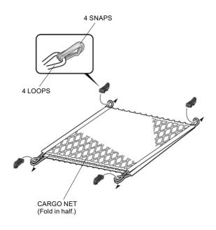
With the opening side of the cargo net facing rearward, secure the four snaps to the hooks in the luggage area.
