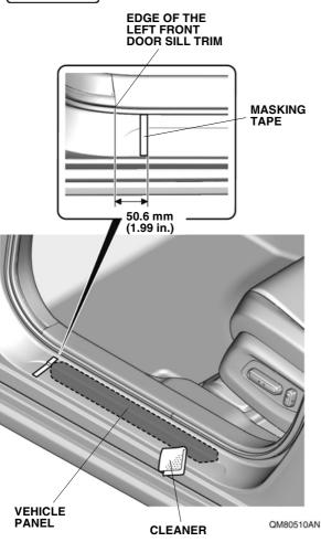
3. Temporarily attach the adhesive backings.
