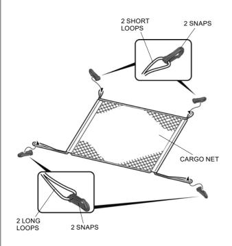
Attach the four snaps to the tie-down hooks and rings.
